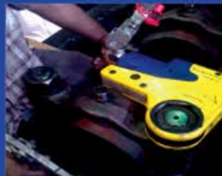
HTW-4X WITH 360°X360° SWIVEL USED FOR TIGHTENING MAIN BEARING NUTS IN DIESEL LOCO SHED
