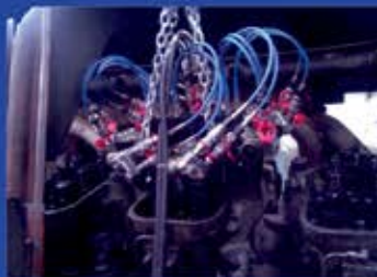
HTW-2T SWYWN No. ALONG WITH FIXTURE FOR TIGHTENING & LOOSENING ENGINE HEAD BOLTS OF ALCO ENGINE
