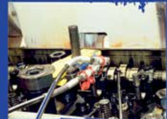
HTW-8D BEING USED ON GM LOCO ENGINE CRABNUT AT DIESEL LOCO SHED SWR, HUBLI
