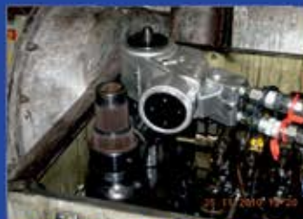
HTW-7T BEING USED FOR CRAB NUT OF WDG4 LOCO FOR TIGHTENING & LOOSENING
